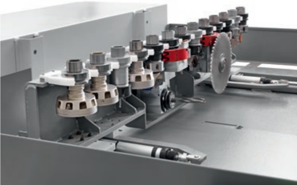
The rack magazine with 13/16 positions provides a simple and functional solution whilst keeping the overall dimensions of the machine as compact as possible.
